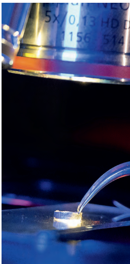
Sample of a metal-organic framework (MOF) compound in glass form. Such components are suitable as starting material for filter membranes that remove carbon dioxide and other hazardous gases during production processes. Photo: Jens Meyer
